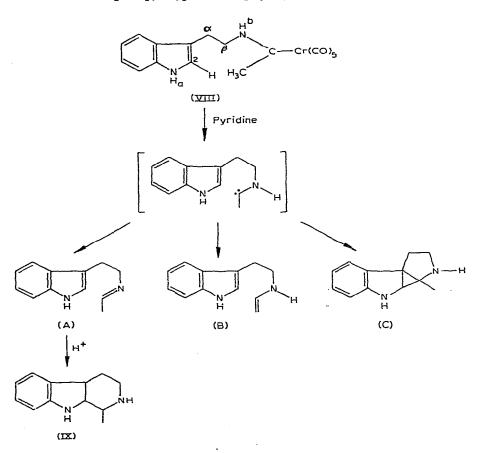
These results show that the base induced displacement of an aminocarbene ligand containing an  $\alpha$ -hydrogen atom attached to nitrogen, results in the formation of an imine as a result of the migration of that hydrogen to the carbene carbon atom. This process is assisted by resonance stabilisation of the product from the aromatic
